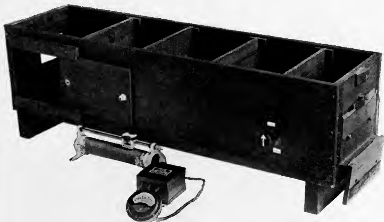
FIG. 2. Eastman model X step tablet sensitometer; for exposing sensitometric strips on all photosensitive materials.
